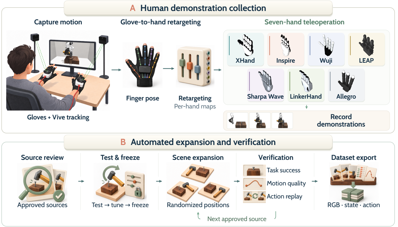
Fig. 3. Collection toolkit. (A) Glove-to-hand mappings enable teleoperation of seven hands using the DexJoCo capture setup [19]. (B) Reviewed demonstrations are expanded into randomized scenes, verified, and exported as RGB, state, and action records.
